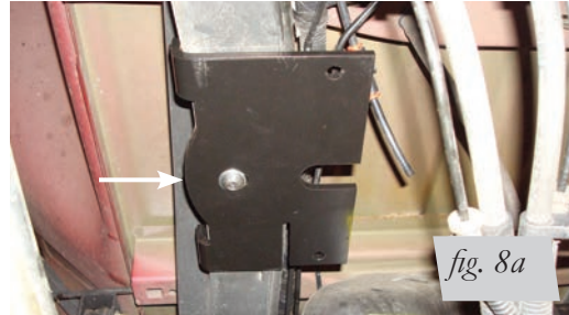
LH (driver's side). Push bracket against frame and torque to 38 lb.-ft. (52Nm).
