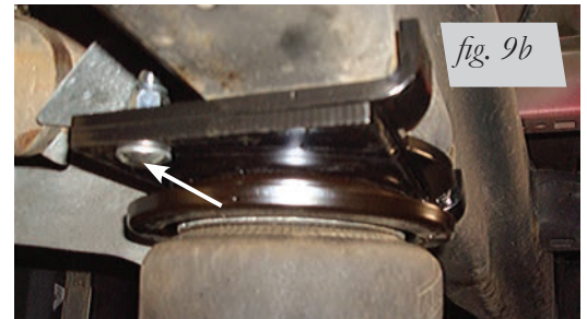
Right hand assembly (passenger's side) attached with carriage bolts (R), flat washers (M) and nylon lock nuts (U). Torque to 31 lb.-ft. (42Nm).
