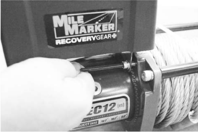
2-5: Screw bolts with control box in the mounting points.
