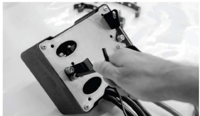
2-3: Install the smaller mounting bracket on the other side.
